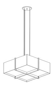
Pull line voltage wires out of the junction box. Make connections between fixture leads and line voltage wires.
