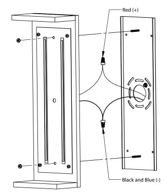
(10) Carefully move the difuser towards the fixture and align the holes in the with the four screws on the shade, then slide the diffuser down to secure the diffuser on the fixture.
