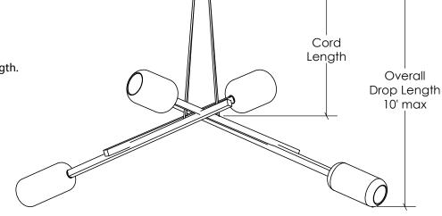
② Use painters tape to indicate the cord length (approximately 16" less than the overall drop length). Make sure all cord lengths are the same length or the fixture will not hang straight.
