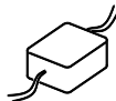
P1, P2, P3 - Hardwire drivers must be housed in a suitable enclosure.
