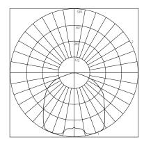
Maximum Candela = 530 Located at Horizontal Angle = 0, Vertical Angle = 24 Fixture specified by using the SKU builder below are subject to increased lead times and minimum order quantities.
