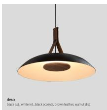
Dimensions: 24" dia., 14.5" Product weight: 7 lb Light source: integrated LED Light output: 2625 Lumens (source) Output based on white shade interior Alternate finishes will reduce lumen output Light color: 2700 K, 3000 K, 3500 K, or 4000 K Color accuracy: 90+ CRI Power usage: 26 W Driver can be housed inside canopy Driver dimensions: 3.38" x 1.63" x 1.08" Dimmable (see driver option)
