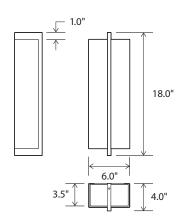
Dimensions: 18" x 6" x 4" Materials: solid wood, polymer Product weight: 2 lb Integrated LED Specifications Light output: 500 Lumens (source) Light color\*: 2700 K or 3500 K Color accuracy: 90+ CRI Power usage: 7 W Dimmable (see driver below) Input voltage: 24 V DC (driver included) Driver location: must be housed in J-box Driver dimensions: 3" x 1.5" x 1" Mounting: ceiling or wall
