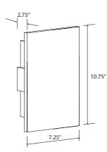
Dimensions: 10.75" x 7.25" x 2.75" Materials: solid wood, polymer, metal option, stone option Product weight: 2 lb (5 lb marble) Light source: integrated LED Light output: 1130 Lumens (source) Light color: 2700 K, 3000K, or 3500 K Color accuracy: 90+ CRI Power usage: 13 W Dimmable (see driver below) Wood grain and stone will vary Specifications subject to change
