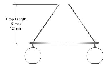
(2) Measure the cord length and use painter's tape to indicate a stop point. Make sure both cord lengths are exactly the same size or the fixture will not hang straight.
