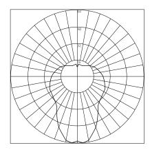
Maximum Candela = 63.79 Located at Horizontal Angle = 90, Vertical Angle = 5
