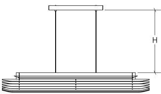
(1) Measure the desired height (H) of the fixture.
