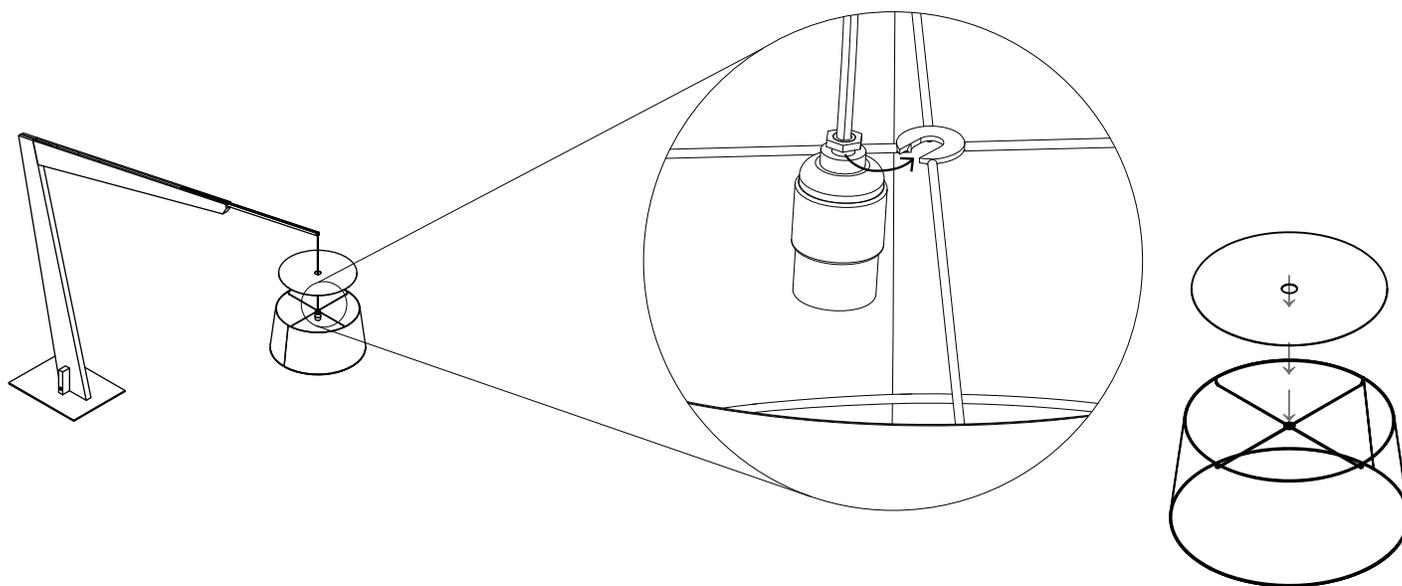
Following shade and top diffuser installation, install the bulb into the socket
