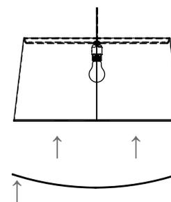
**NOTE:** For uninstallation of lower diffuser gently lift up one edge of the lower diffuser and carefully bend the diffuser until it can be removed from the bottom of the shade assembly.
