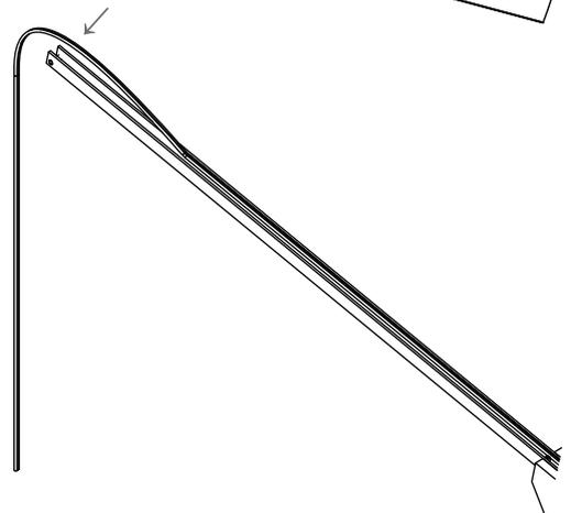
**11.** Adjust the height that the shade hangs by winding the cord around the studs in the groove in the top of the body.
