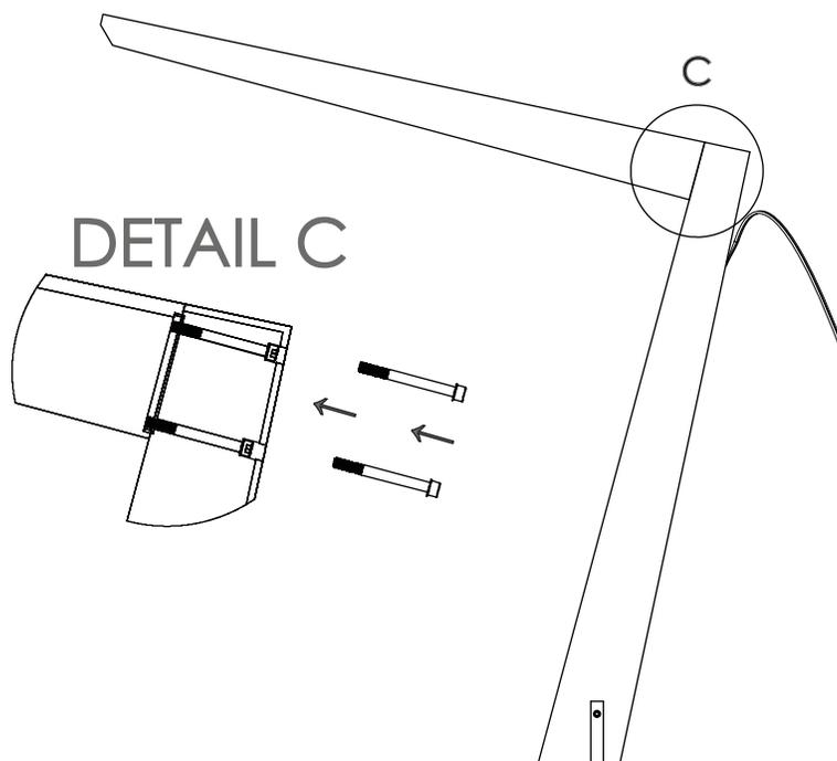
4. With the body components now securely fastened, press the wire and cord stock into the groove covering the joint.
