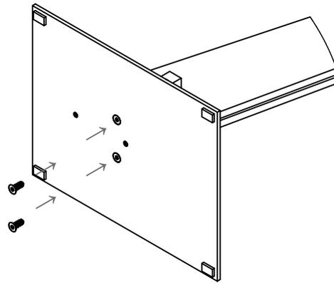
**6.** Following the installation of the fasteners in step 6, insert the two wood screws and tighten them.
