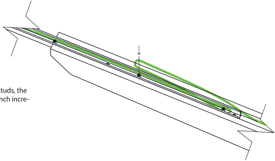
**12.** By wrapping the cord around different studs, the height of the shade at can be adjusted in 8 inch increments.
