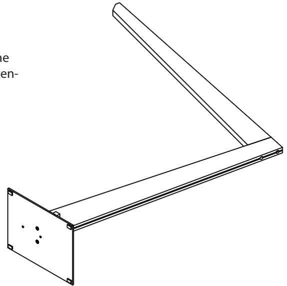
**5.** Once the base is in position, insert the two 1/2-13 flat head socket screws and tighten using a 5/16" hex key.
