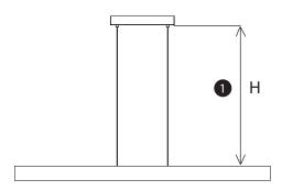
Feed the cables through the following parts in this order: canopy thumbnut, canopy, mounting plate bracket, and strain relief tab. After feeding the cable through the strain relief tab, tie a strain relief knot using the black mesh of the cable while maintaining the desired height (H).
