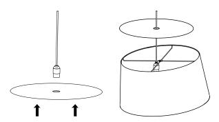
Following shade and top diffuser installation, install light bulb into socket.
