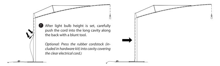
(Stretching the rubber cord can make it easier to press into the cavity, but will effect its overall length. Excess rubber cord can be trimmed easily with scissors.)
