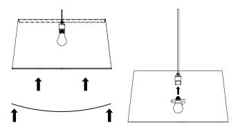
**NOTE:** To remove lower diffuser, gently lift up one edge of the lower diffuser and carefully bend the diffuser until it can be removed from the bottom of the shade assembly.
