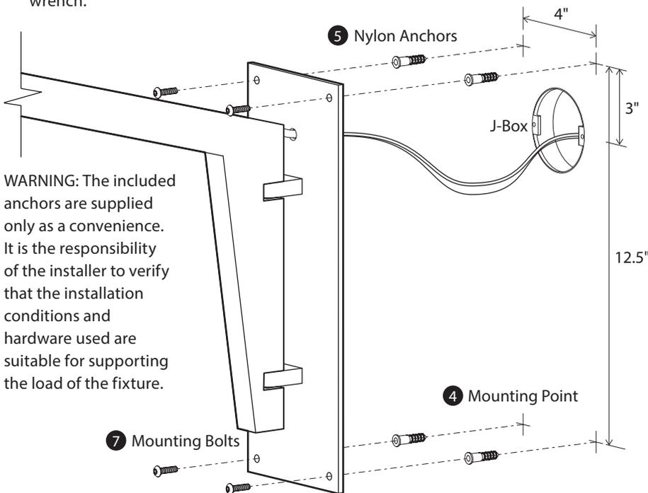
**WARNING:** The included anchors are supplied only as a convenience. It is the responsibility of the installer to verify that the installation conditions and hardware used are suitable for supporting the load of the fixture.
