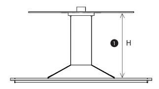
Feed the cables through the following parts in this order: canopy thumbnut, canopy, mounting plate bracket, and strain relief tab. After feeding the cable through the strain relief tab, tie a strain relief knot using the black mesh of the cable while maintaining the desired height (H).
