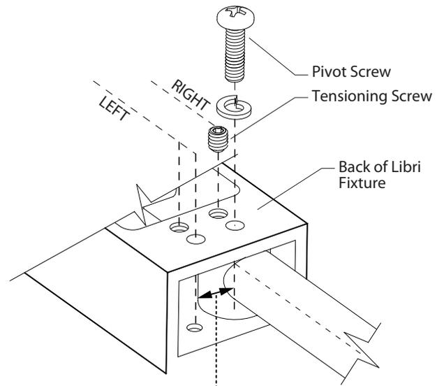
To change the orientation, remove the pivot screw and the tensioning screw. Slide the arm and washer over to the other side and line up the holes. Screw in the pivot screw to secure the arm. Taking care not to pinch the wires running through the arm. Tighten the tensioning screw to the desired tension.
